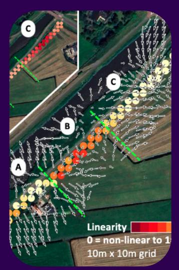
GEORISK MONITOR is a cloud-based web platform that empowers cities to proactively manage the risks posed by ground deformation to civil infrastructure. By transforming satellite data into actionable geological insights, the platform enables detailed monitoring of land displacement and infrastructure stress at a city-wide or site-specific scale.
